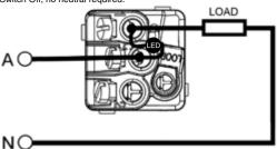
4. LED On, Switch Off, using neutral.
