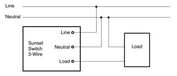
\*NOTE: applications using small fluorescent loads, or other loads, which are sensitive to leakage current, may require a load correction device (Cat. No. 31CAP).
