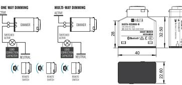
\* Maximum 8 Remote Switches \* Max 3x units per standard wall plate
