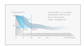
With the Turbo function the motor and fan work at a higher frequency, so you can enjoy a cool room within a much shorter time.
