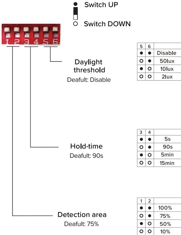
Definition of the ambient brightness; only when the ambient brightness is lower than the preset specific lux amount, the sensor will work; when it's preset as "Disable" the sensor works everytime it detects motion regardless of the ambient brightness.
