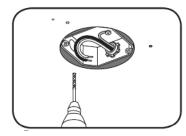
2. Mark and drill holes in mounting surface and install plug anchors.
