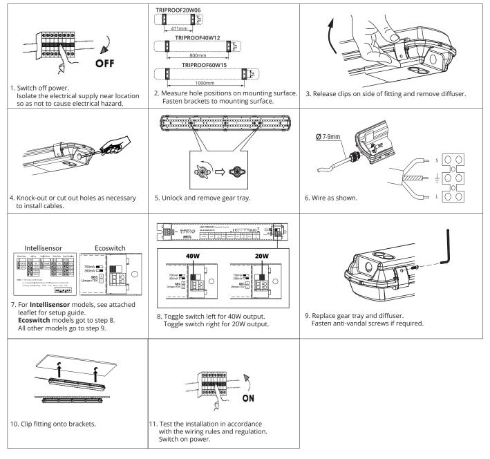
Installation of the product must be carried out by a licensed electrician, in accordance with these instructions and relevant Australia Standards or local regulations.
