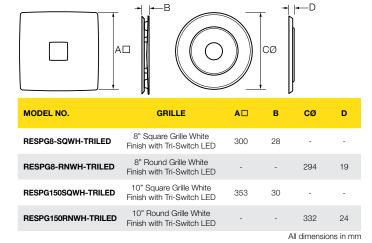
INPUT BEAM LUMENS **COLOUR TEMP** MODEL NO. GRILLE **POWER** ANGLE (LM) (W) (°) RESPG8-SQWH-TRILED Square 1000 12 3000/4200/6000 180 RESPG8-RNWH-TRILED 800 3000/4200/6000 180 RESPG150SQWH-TRILED 1000 3000/4200/6000 RESPG150RNWH-TRILED Round 3000/4200/6000 800 180
