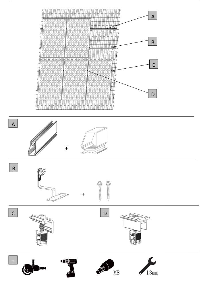
STEP 1. Remove or slide the tile from the roof girder slightly, and place the roof hook on the wooden rafter (refer to the picture below), Fix the roof hooks using two wooden screws. Grind tile as required and replace. (Recommended Torque12-14N.M)
