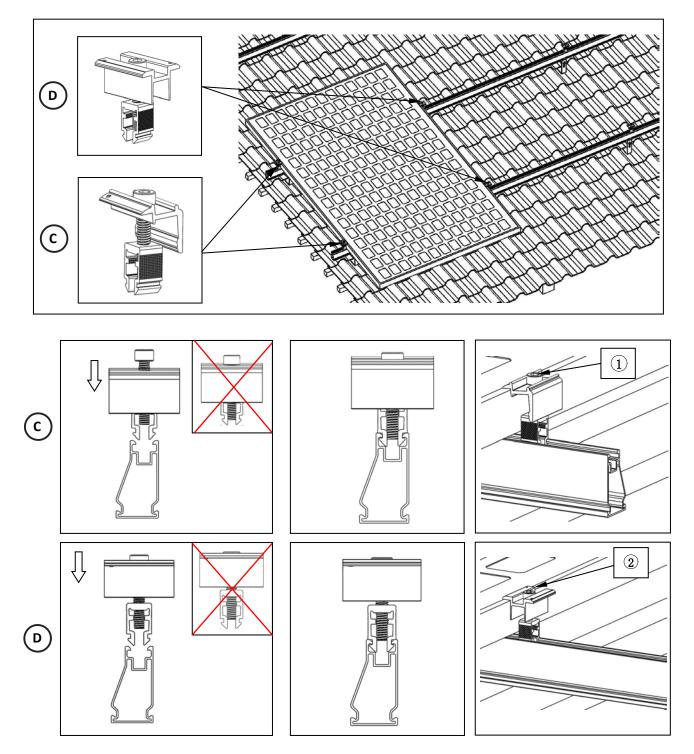
Attention: 1.Ensure the PV Module clamps are pushed up against the solar panel.
