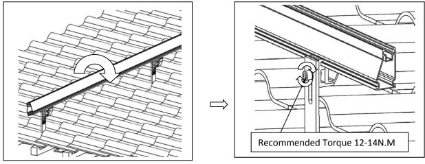
STEP 3. Join the rails by sliding the rail joiner into the rail
