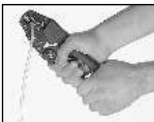
When the connector and cable are fixed, the final crimping can be done with a comfortable two-hand grip.
