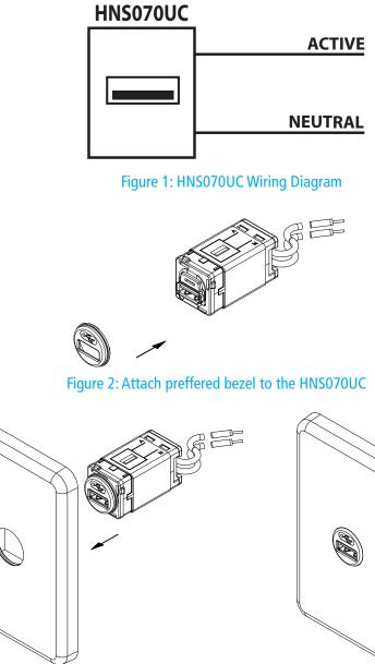
Figure 3: Attach HNS070UC to the wall plate
